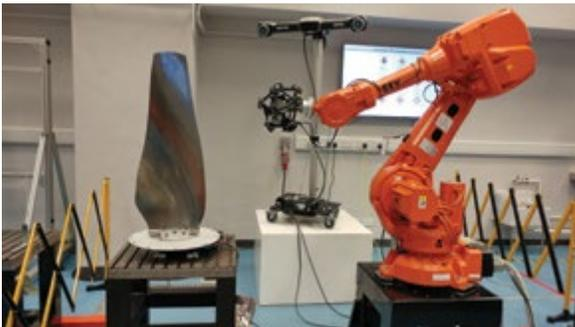
Defect identification using robot and 3D camera
